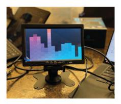
DAV offers students two tracks. The original track, Digital Audio Visualizer, requires members to interface their FPGA with a microphone and perform the Fast Fourier Transform (FFT) to create a histogram of frequencies. In the second track, Digital Design, Architecture, and Verification, members create a game on the FPGA. Members will learn about serial communication protocols like I2C to achieve communication between their FPGA and a peripheral game controller.
