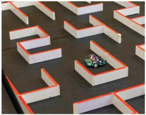
IEEE at UCLA's longest-established advanced project, Micromouse, challenges students to develop their skills in circuit design, sensor data acquisition, signal processing, control systems, and algorithms in order to create a maze-solving robot. Over the school year, teams design, build, and program small autonomous robots and use them to navigate and solve a 16x16 cell maze. Teams compete for the fastest time by combining search and speed runs.
